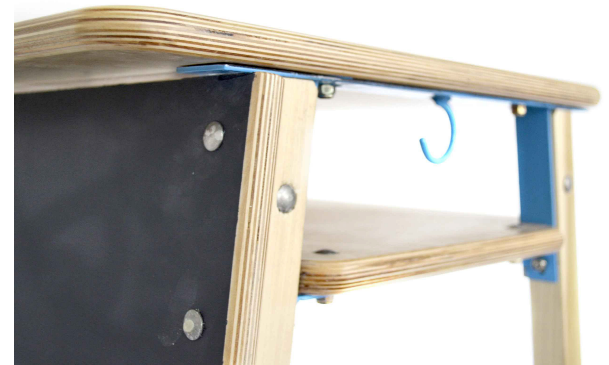
FRONT DESK CONNECTION SHOWING CHALKBOARD EDGE AFTER ROUTING AND BOLT HEADS TO SURFACE
