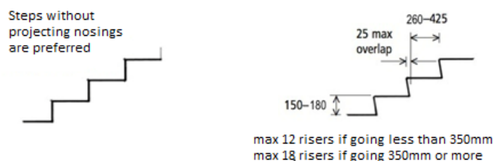
Figure 24: Profile of stairs (Source: Centre for Accessible Environments and RIBA 2004)
