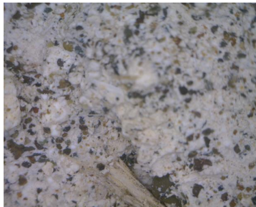
Fig. 11. Presence of organic materials in the base layer and the painted layer
