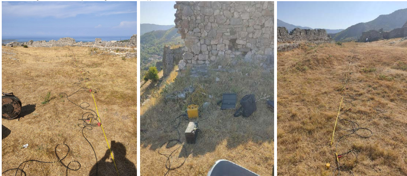
Figure 2 Aspects of the work carried out on the construction site using the MASW method
