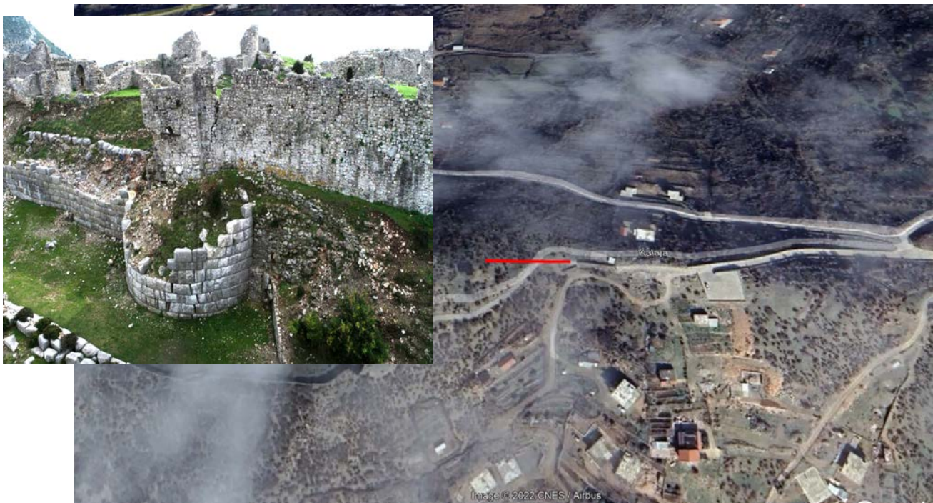
Figure. 1 Ortofoto of the area of the construction site. The red line represents the position of the seismic line through which we performed the seismic study using the MASW method
