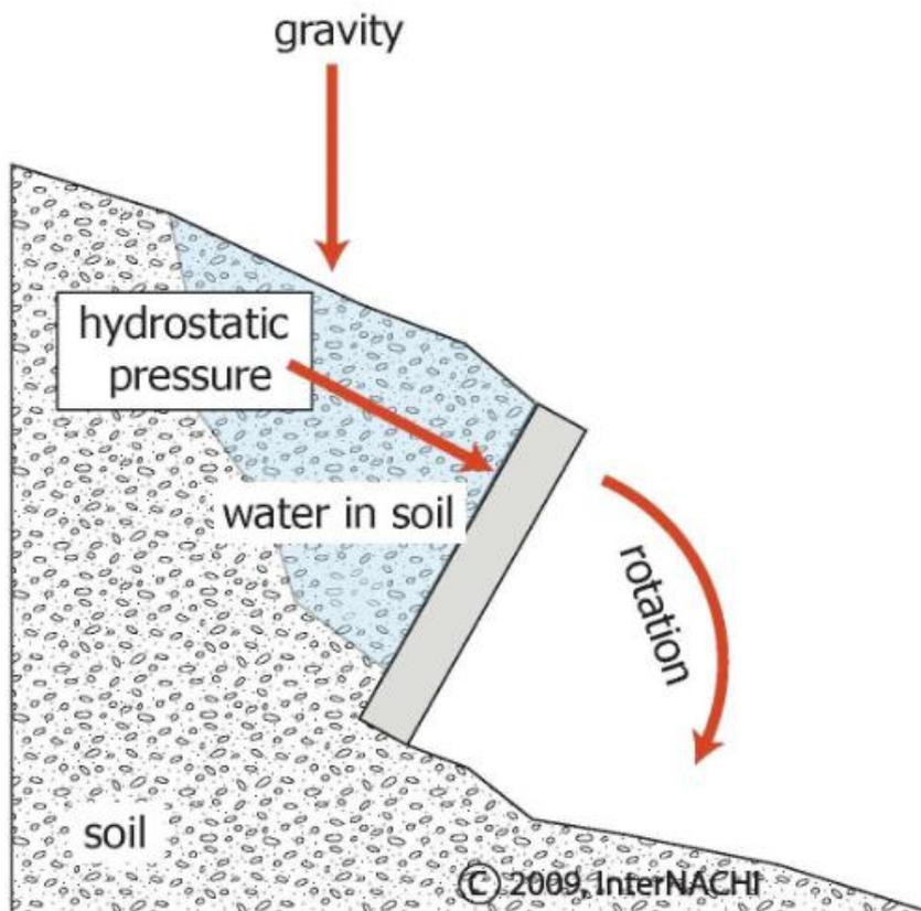
6. Loss of the bearing capacity at the base of the foundation, regardless of the fact that the exposed area may not be the true base of the retaining wall, there is a loss of the bearing capacity of this area, this is also reflected in local damage to the retaining wall near the foundation, something that has put the entire retaining wall in more difficult conditions and may be the main reason for the advancement of the further movement of this part of the wall.
