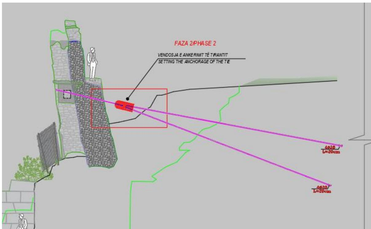
We should also consider placing a recorder when tightening the tie rod in order to check and accurately reach the value we need in the horizontal direction (550 kN)
