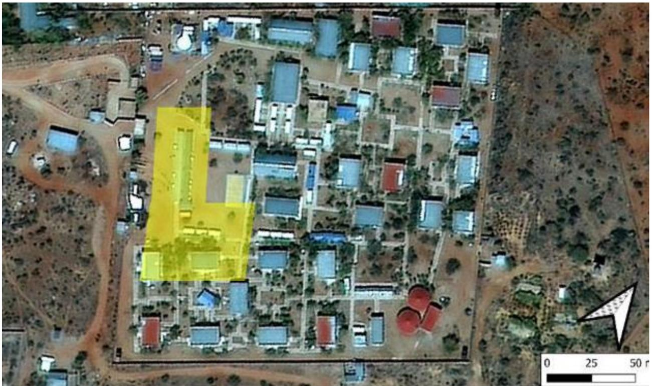
The main distribution board is situated in the north-west side corner of the compound, 50 meters away from the north side of the area highlighted in yellow. The structure shall be an elevated mounting structure with a height of 5 meters.
