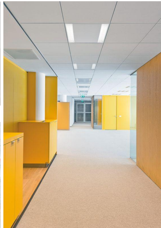
Acoustic Panelling Type 8 Perforated Mineral Fiber Ceiling Tiles - Common Areas / Learning Studios
