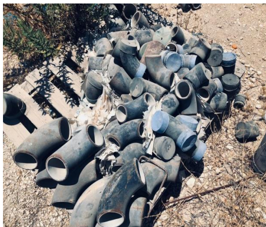
Bends and Elbows need cleaning and insulation. The damaged ones have to be excluded.
