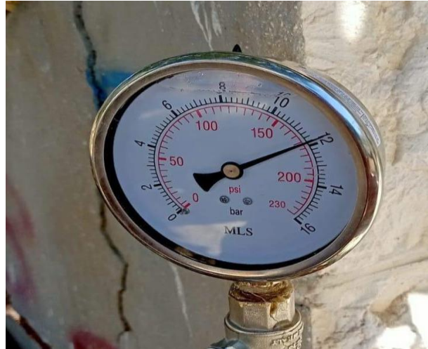
Pressure Test No. 1: 11.9 bar. reading after the pressure test.
