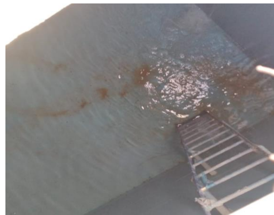
Tank during the filling- 25% filled. No Water leakage through floors, walls, or wall-floor joints.
