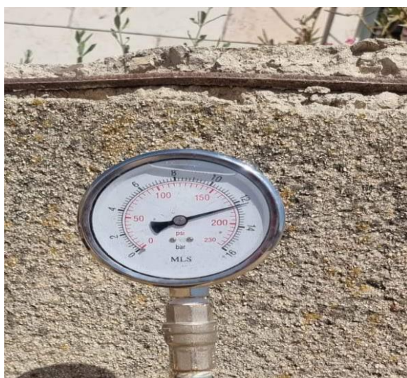
Pressure Test No. 1: 12.1 bar reading once pressurized
