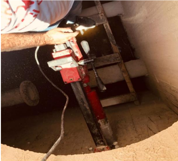
Core Test for Concrete Chamber #5
