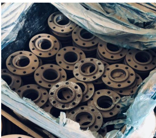
Flanges need cleaning using sand blasting
