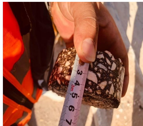
Core Test for Asphalt #1 – 4.40 cm
