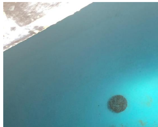
Tank during the filling- 50% filled. No Water leakage through floors, walls, or wall-floor joints.
