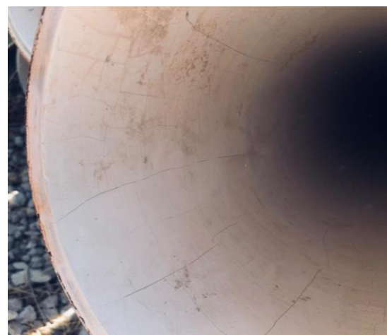
Steel Pipes. The pipes with cracks in the cement lining must be excluded, less than 20%
