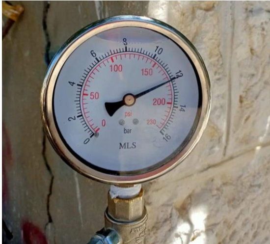
Pressure Test No. 2: 12.0 bar reading once pressurized
