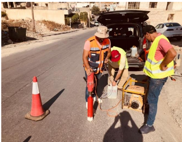
Core Test for Asphalt #10 – Taking Samples
