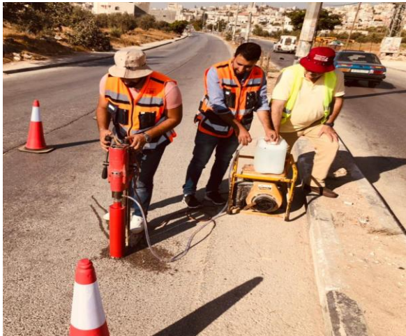
Core Test for Asphalt #1 – Taking Samples
