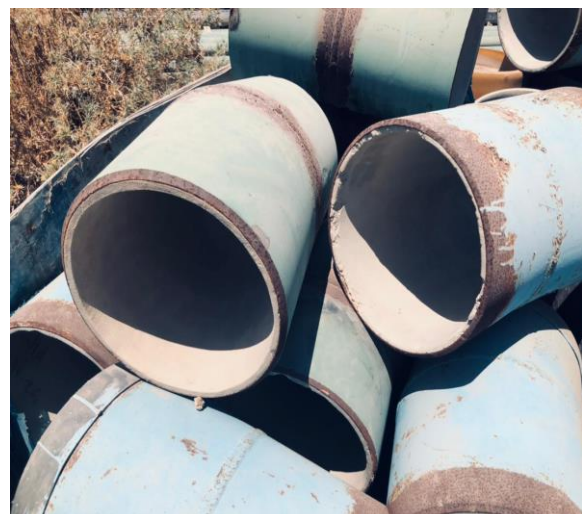
Will need some repair and insulation before use
