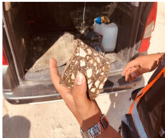
Core Test for Asphalt #10 – 7.10 cm
