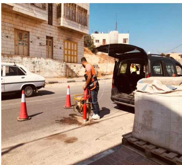
Core Test for Asphalt #30 – Taking Samples
