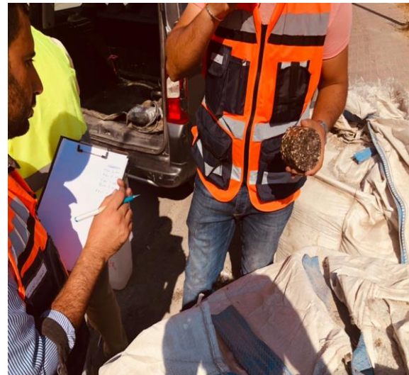
Core Test for Asphalt #30 – 8.20 cm
