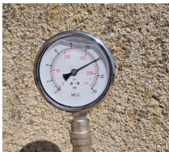
Pressure Test No. 1: 11.9 bar. reading after the pressure test.
