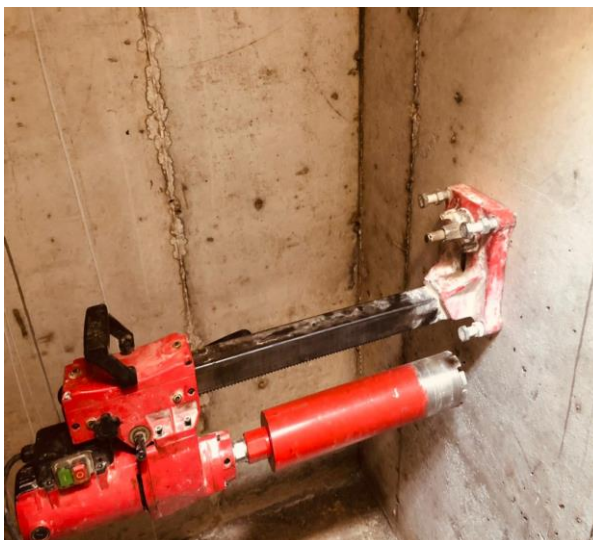
Core Test for Concrete Chamber #1
