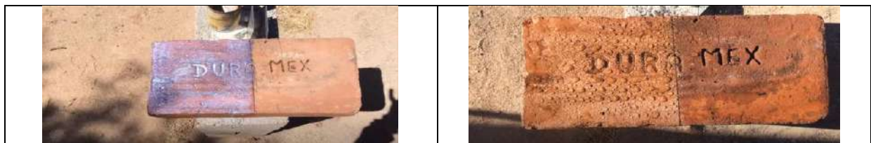
Fig. 31: Application of hydrophobic solution to adobe bricks
