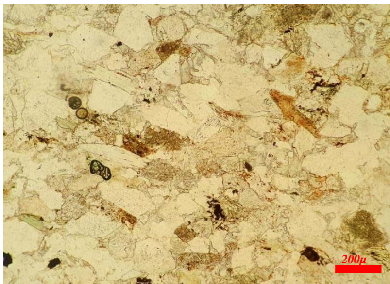
Figure 30. Detail of Figure 18, biotite and chlorite formations. Thin section of the sand sample from the foot of the Kurçaj bridge. Planar polarized light and permeable, without analyzer
