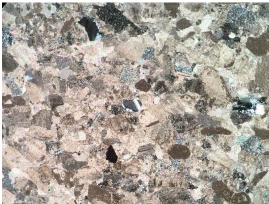
Figure 13. Plagioclase subrounded particle located between carbonate particles. 5D sample, light penetrated by analyzer
