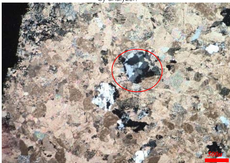
Figure 18. Polycrystalline quartz with straight boundaries between crystals (red circle). 5D sample, light penetrated by analyzer.
