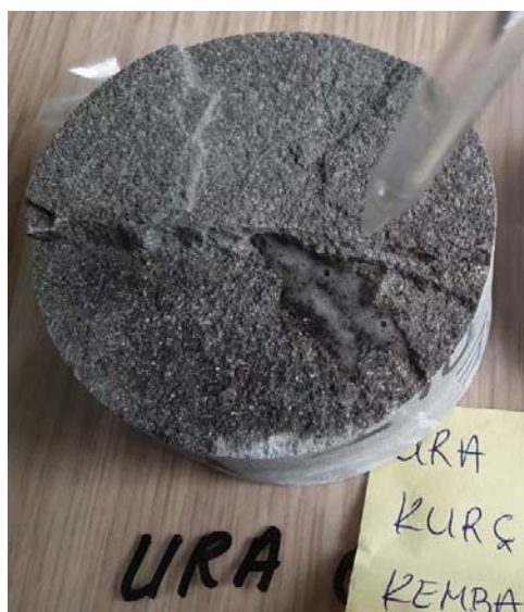
Figure 22. View of the sand sample from the foot of the Ottoman bridge Kurçaj reacting with 10% HCl acid.
