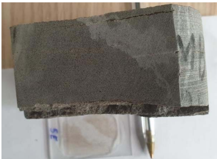
Figure 23.. Irregularly shaped calcite vein that traverses the sand sample from the foot of the Ottoman bridge, Kurçaj.
