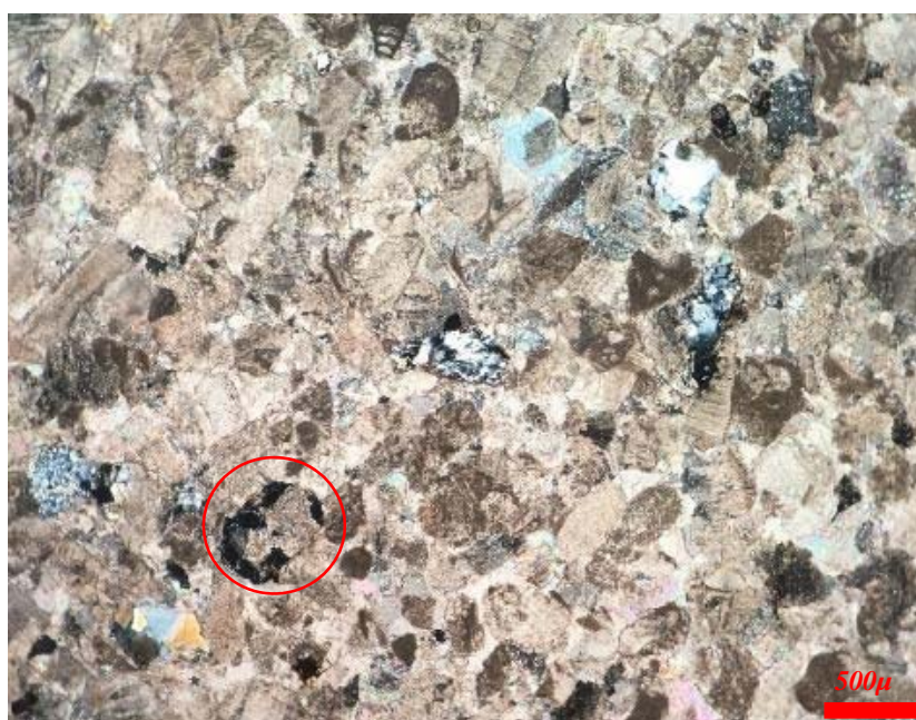
Figure 16. Fragments of well-preserved to partially altered igneous rocks (red circle). 5D sample, light penetrated by analyzer.
