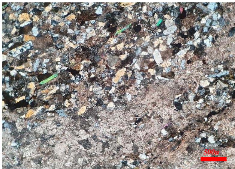
Figure 27. Muscovite leaflets are oriented subparallel to the calcite vein. Thin section of the sand sample from the foot of the Kurçaj bridge. Planar polarized light and permeated, with analyzer.
