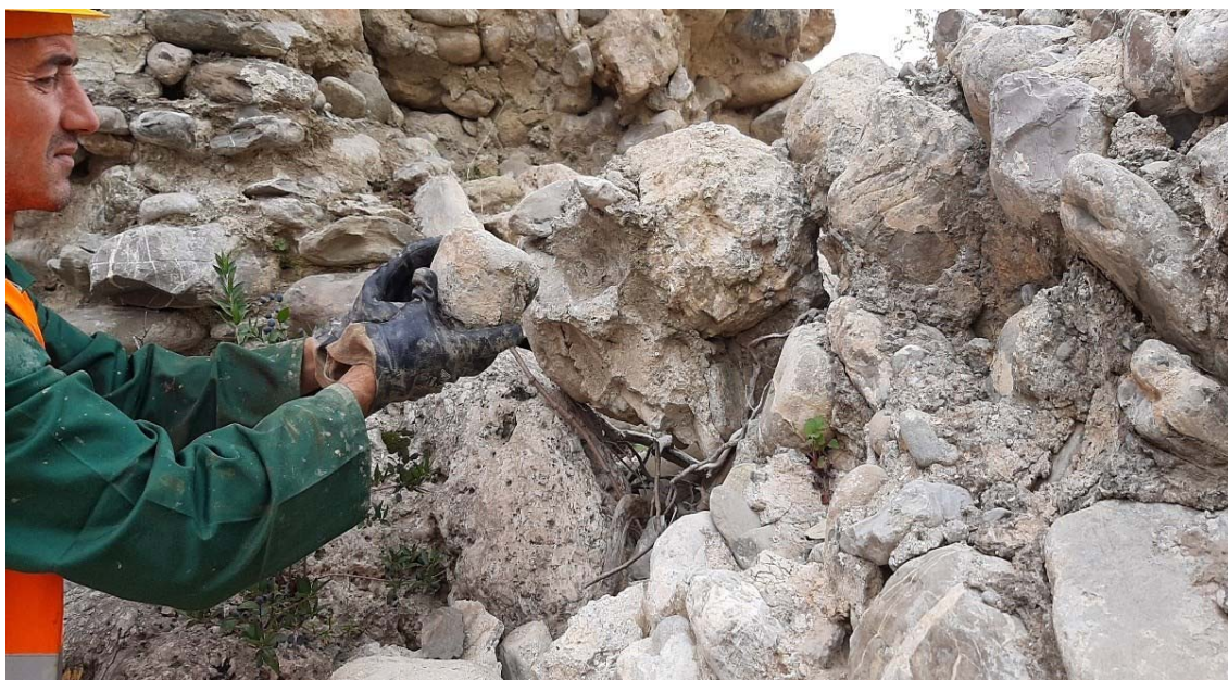
Figure 7: Recovery of Limestone sample at the small arch of the bridge by the village of Zgerdesh.
