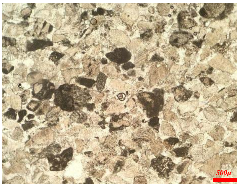
Figure 10. Biogenic material which forms a supporting granular texture of rock. 5D sample, light penetrated without analyzer
