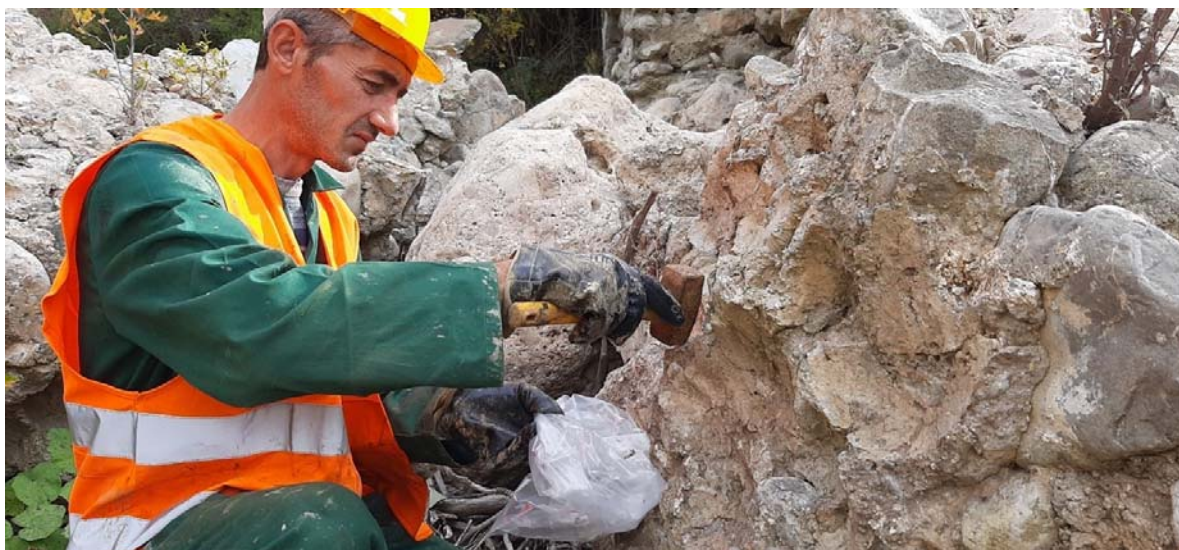
Figure 8: Recovering Mortar sample at the small arch of the bridge.
