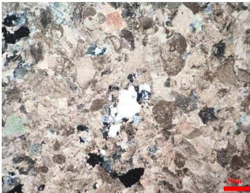
Figure 17. Combination of monocrystalline quartz with polycrystalline. 5D sample, light penetrated by analyzer.
