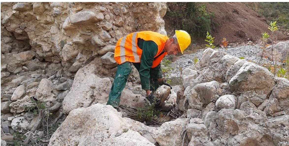
Figure 6: Recovering Sandstone sample at the foot of the bridge by the village of Zgerdesh.
