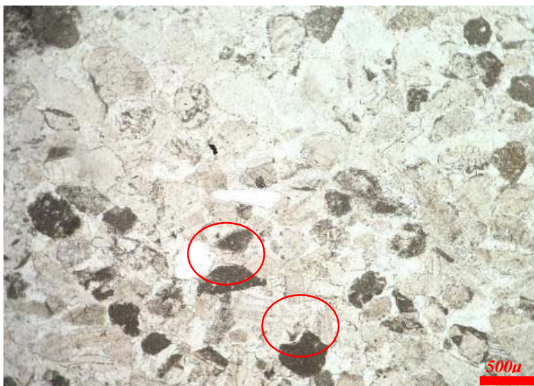
Figure 11. Carbonate material represented by fragments of fauna and subcondytic micritic particles (red circles). 5D sample, light penetrated without analyzer.
