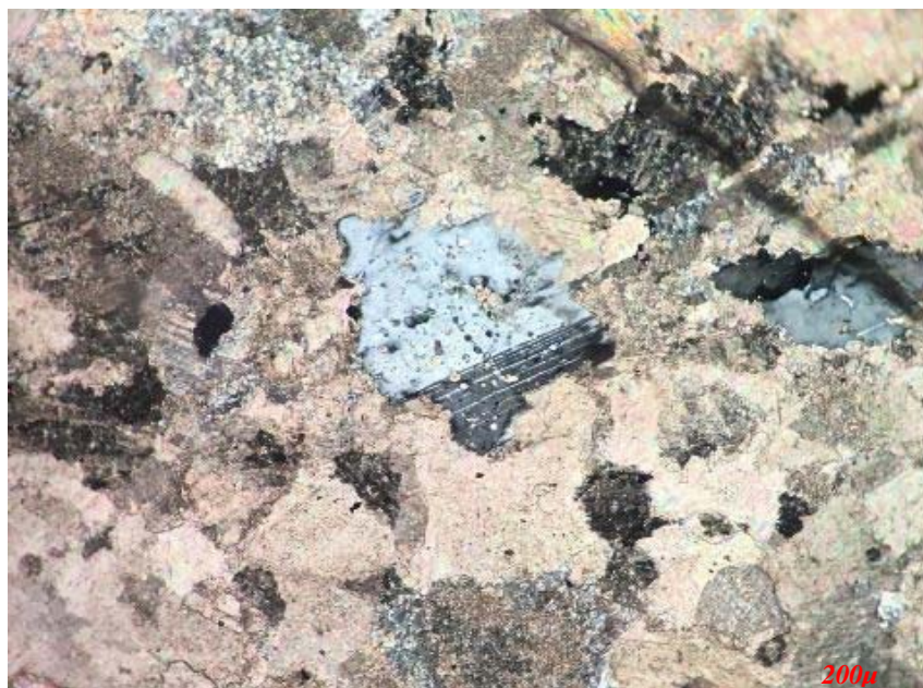
Figure 19. Plagioclase crystals which appear in the early stages of alteration. 5D sample, light penetrated by analyzer.
