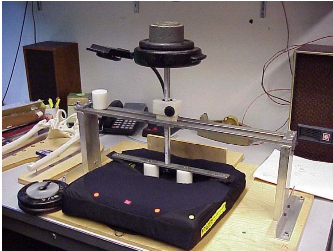
Loaded contour depth stand & jig in use
