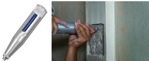
Fig. 29 –Schmidt hammer concrete evaluation
