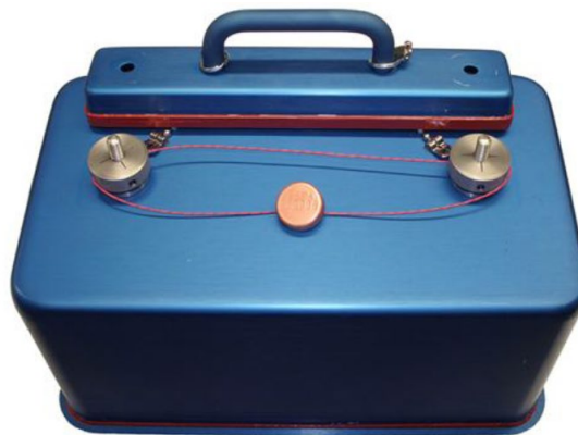
Figure 1. CAPS seal shown attached to an electronics housing. (The handle and seal covering are placed over the seal and seal wire to prevent inadvertent damage.)
