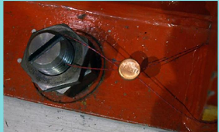
**Example:** the multi-stranded wire is strung through the bolt, so the bolt cannot be removed without removing the wire. The loop material must show evidence of tampering, even if someone tries to fix it.
