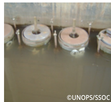
Improper CBR Soaking - the water level should always be maintained above the top of specimen.
