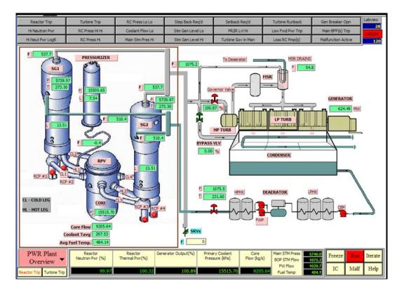
Figure 2.3. Simulator GUI Example: Cassiopeia Technologies Inc. 2007
